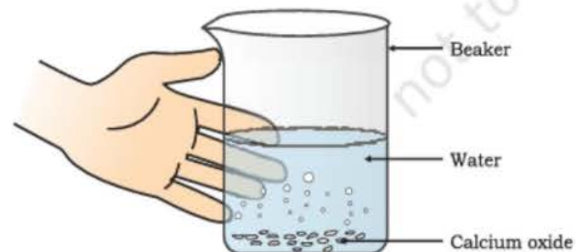
Figure 1.3 Formation of slaked lime by the reaction of calcium oxide with water
